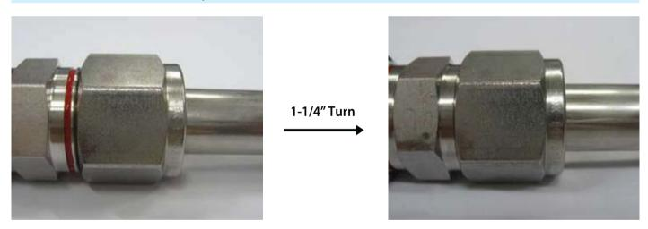
The red color on body identifies DK-LOK VR Series Tube Fittings. It is disappeared by the nut when the fitting's make-up is completed with 1 1/4 turns beyond finger tight position.
