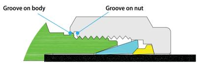
The Patented Groove constructed both on Stainless Steel DK-LOK Tube Fitting Nut and Body locks the Nut up on the Body mechanically at 1 1/4 turns beyond the finger tight.
